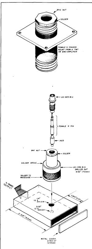
fig. 2. Simple X-band waveguide amplifier mount uses WR-90 waveguide and BNC connectors modified as shown. An alternative female N chassis mount may be made from a TWT or BWO amplifier. No need to drill out the connector in this design.
